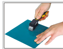
step 1: make grid cutting on surface
